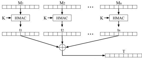
1. Compute HMACs on each individual message.  $t_i = HMAC(K, M_i)$ , for  $1 \le i \le n$ .
